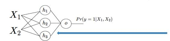
Hidden layers are also called "dense" layers or "fully connected" layers
